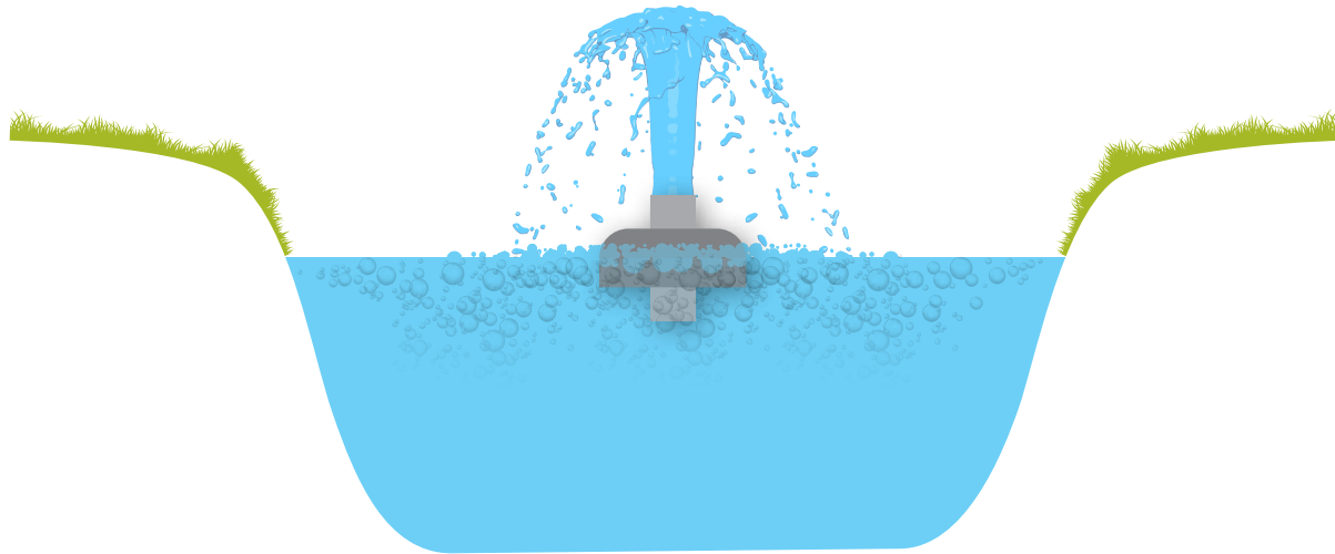
Example of a surface fountain-type aeration system. © EOS Ecology
